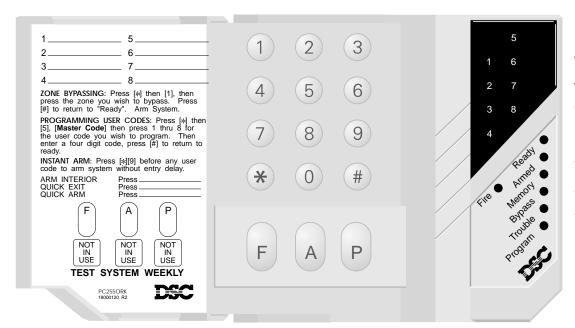
Zone Lights 1 to 8 indicate zone activity. With the system disarmed, the Zone Lights will come ON to indicate when zones are active, and the Zone Lights will be shut OFF to indicate that zones are secure.
